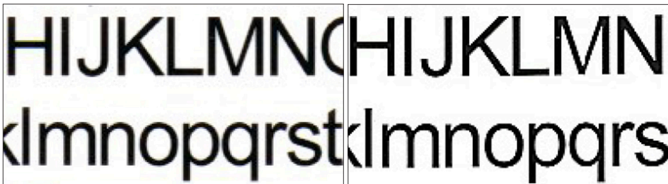
Canon (left) and HP (right) fonts in Standard/Normal resolution settings, at 300-dpi resolution. Note the pronounced stair-stepping in diagonal lines and curves (J, M, s, etc.) on the HP's output.
