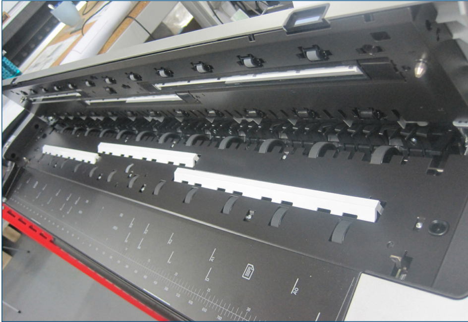
HP DesignJet T830 MFP scanner design employs a staggered array of RGB LEDs.
