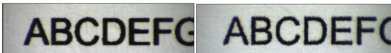
6pt copied text in High 600 dpi (Canon, left) and Best 600 dpi (HP, right); character definition has improved on both model's output, but Canon's text is much bolder, smoother and more distinct when viewed under magnification.
