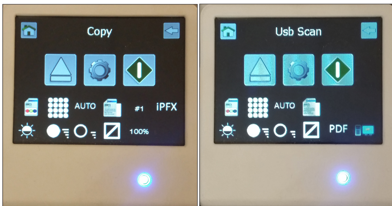
Canon TM-300 MFP L36ei Control panel displaying its Copy screen (left) and Scan to USB (now supported with the L36ei scanner) screen (right).
